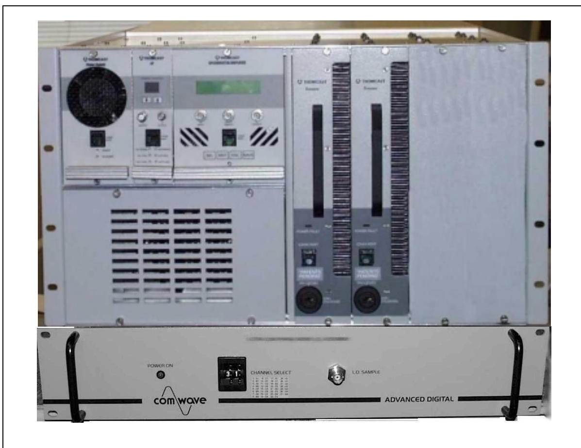
Figure 1: SDA2500C transmitting system (SD2500C with Agile Synthesizer Drawer).
