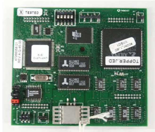
Figure 1 47266058 PCB Top Side View
