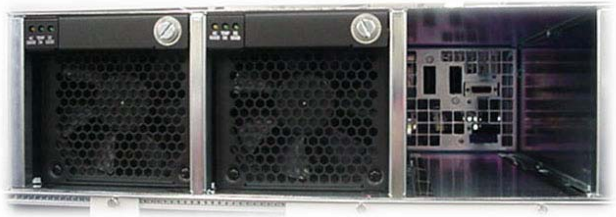
Front-End Power Supply
