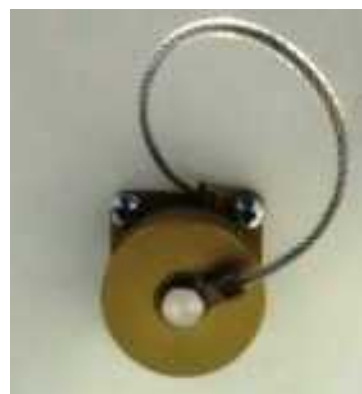
Detail of fibre connector on base of enclosure
