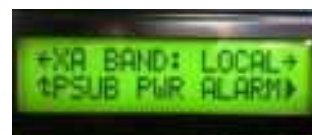
Example of system status with active alarms
