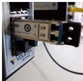
SFP module uninstalled
