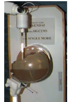
Figure 1. SAR Test Set-up
