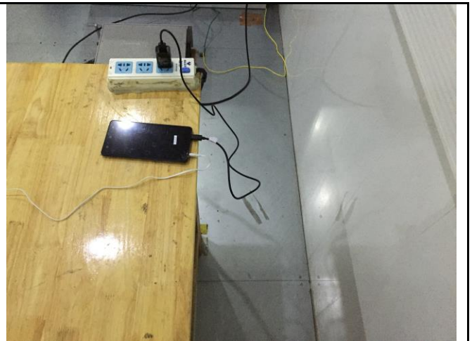
Conducted Emissions Test Setup Side View
