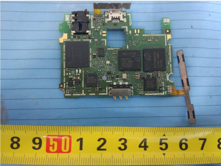
EUT – Main Board Bottom Shieding off View
