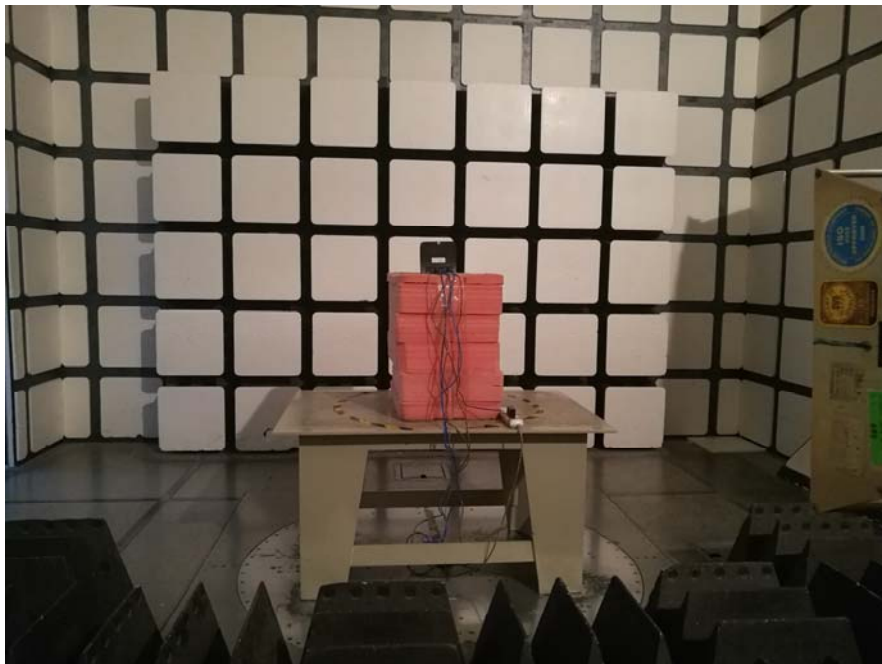
Radiated Emissions View (Above 1 GHz)
