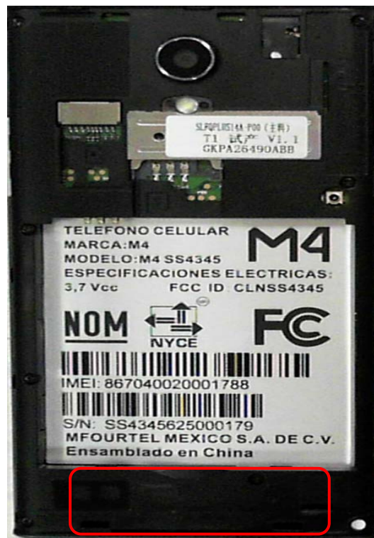
GSM/DCS/UMTS Antenna View
