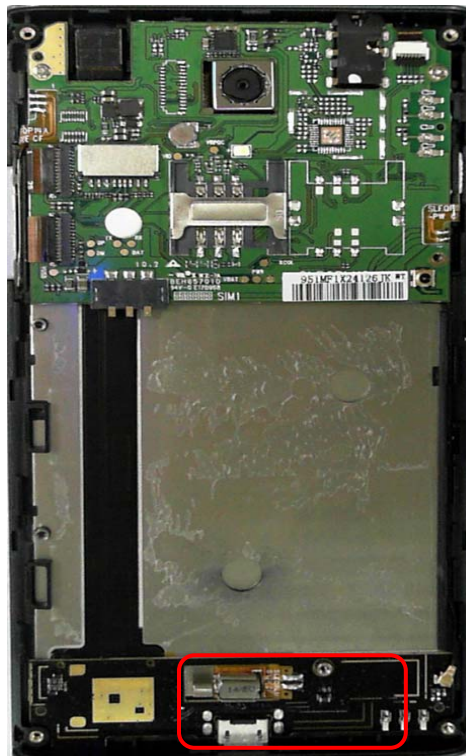
GSM/DCS/UMTS Antenna View
