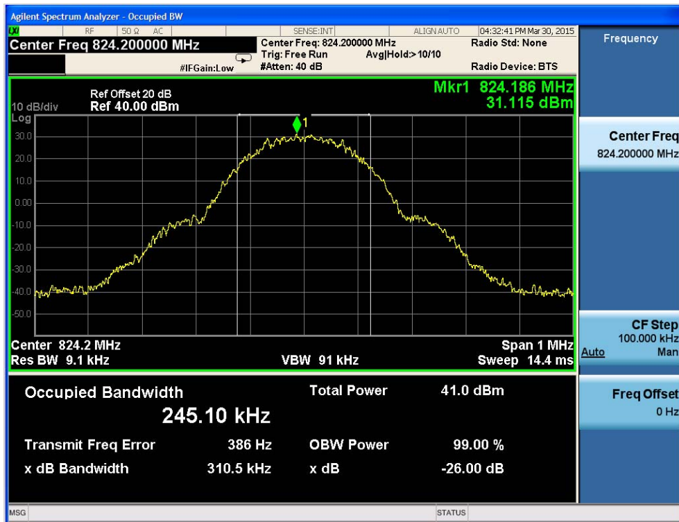
Fig.1 GSM850-CH128 Occupied Bandwidth
