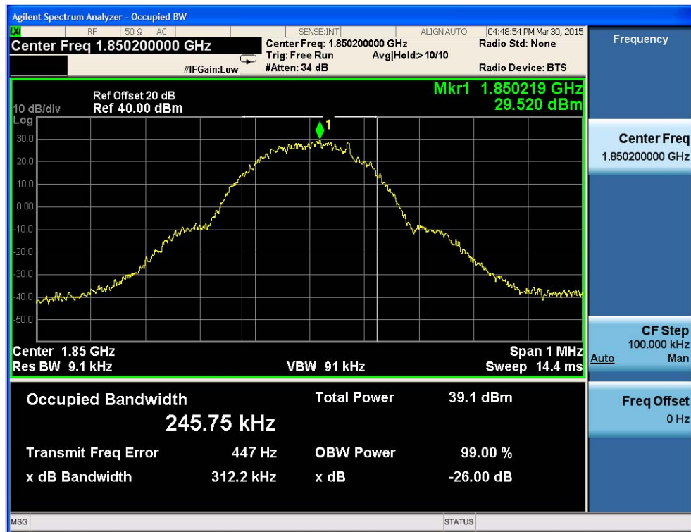
Fig.4 GSM1900-CH512 Occupied Bandwidth
