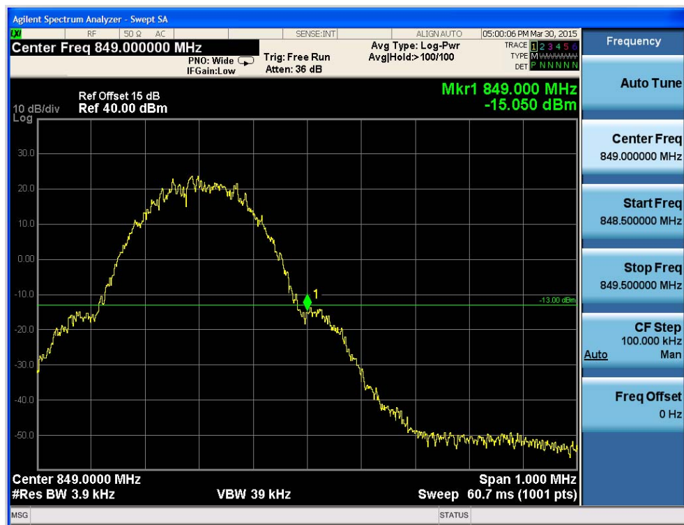
Fig.26 GSM850-CH251 Band Edge Compliance
