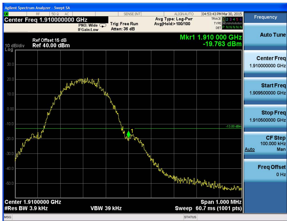
Fig.28 GSM1900-CH810 Band Edge Compliance
