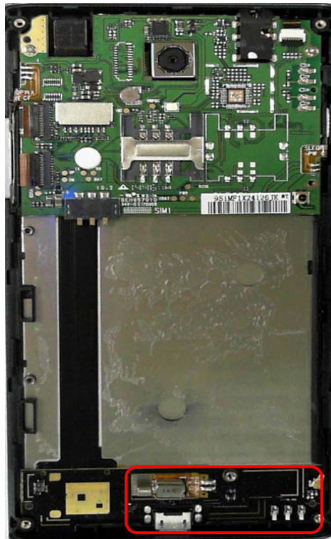
GSM/DCS/UMTS Antenna View
