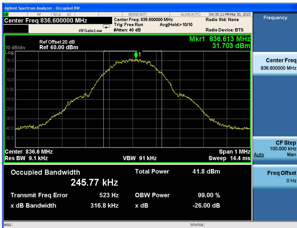
Fig.2 GSM850-CH190 Occupied Bandwidth
