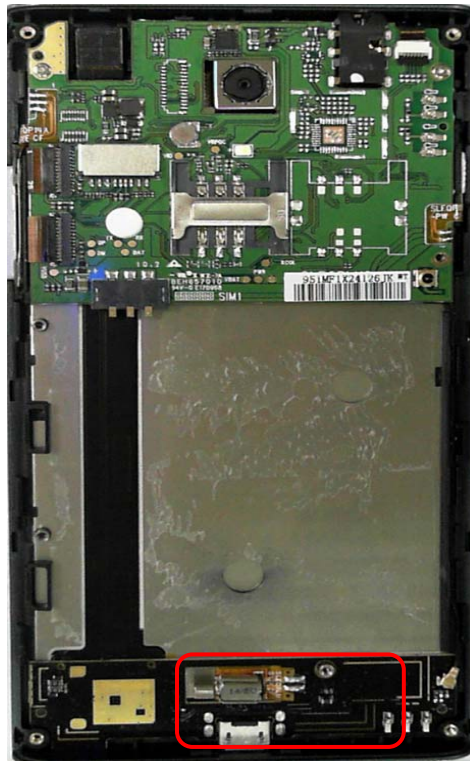
GSM/DCS/UMTS Antenna View
