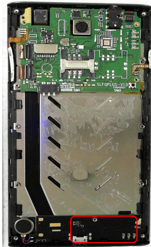
GSM/DCS/UMTS Antenna View
