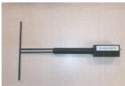
Figure 1 – Satimo COMOSAR Validation Dipole
