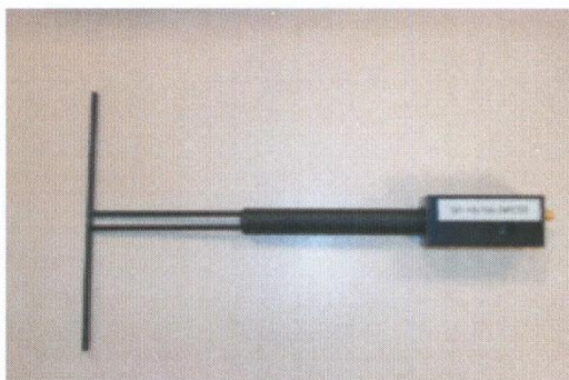
Figure 1 – Satimo COMOSAR Validation Dipole
