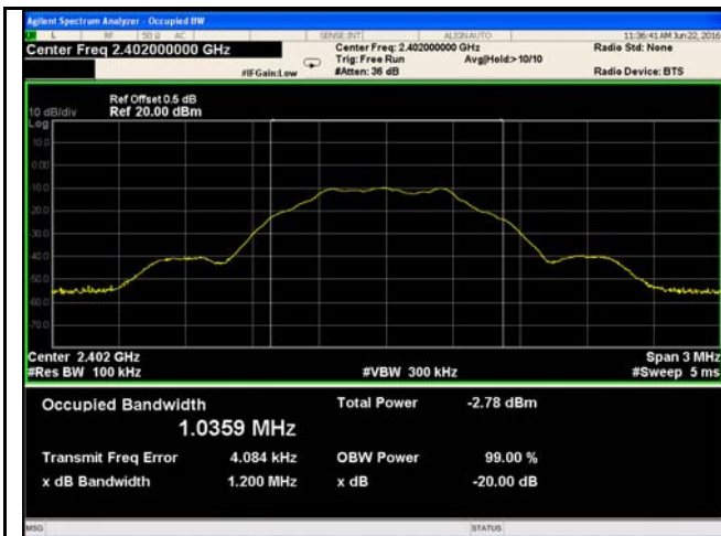
6dB Bandwidth - Low CH 2402
