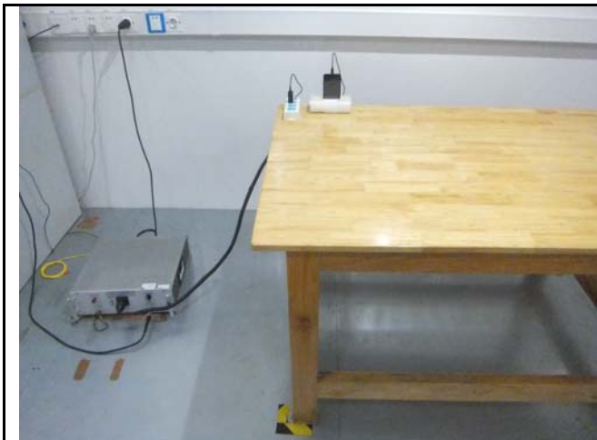
Conducted Emissions Test Setup Front View
