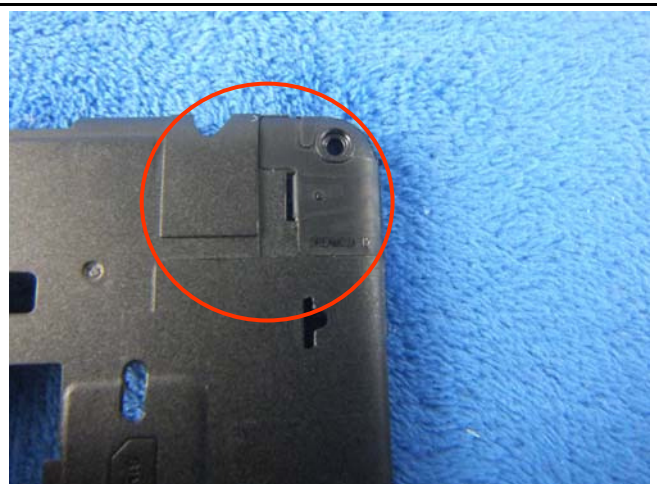
WIFI/BT/BLE/GPS - Antenna View
