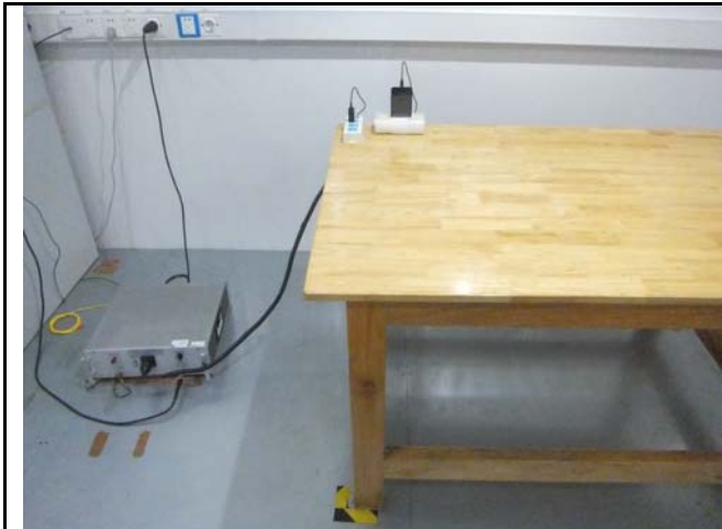
Conducted Emissions Test Setup Front View
