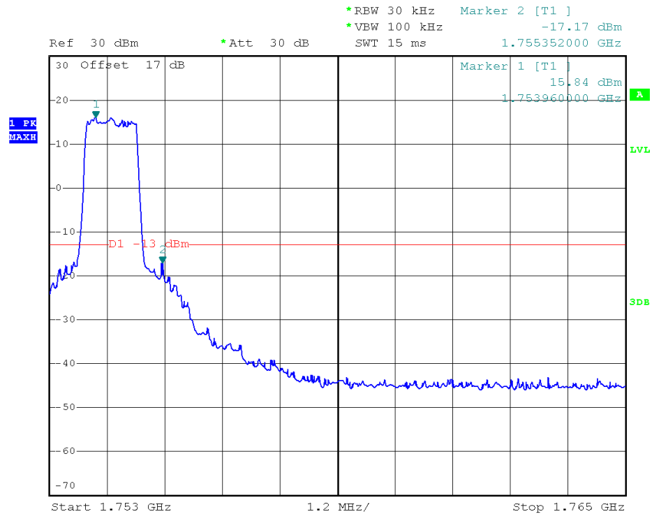
Higher Band Edge Plot for QPSK-RB Size 6, RB Offset 0
