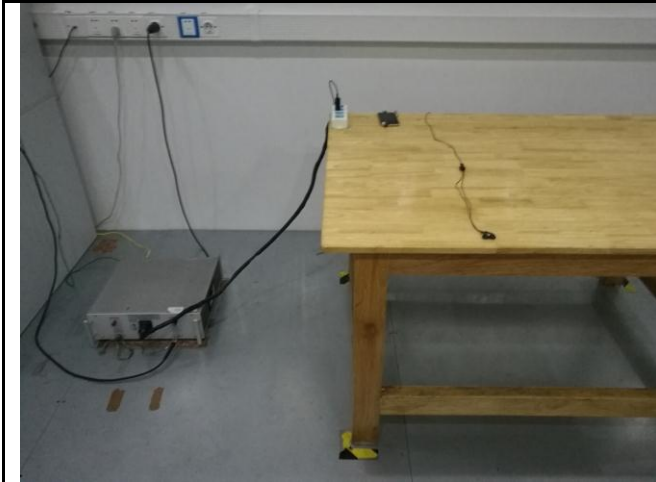
Conducted Emissions Test Setup Front View
