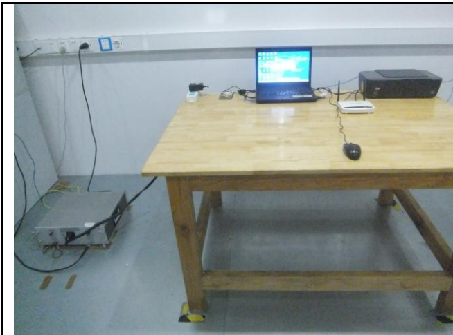
Conducted Emissions Test Setup – Front View
