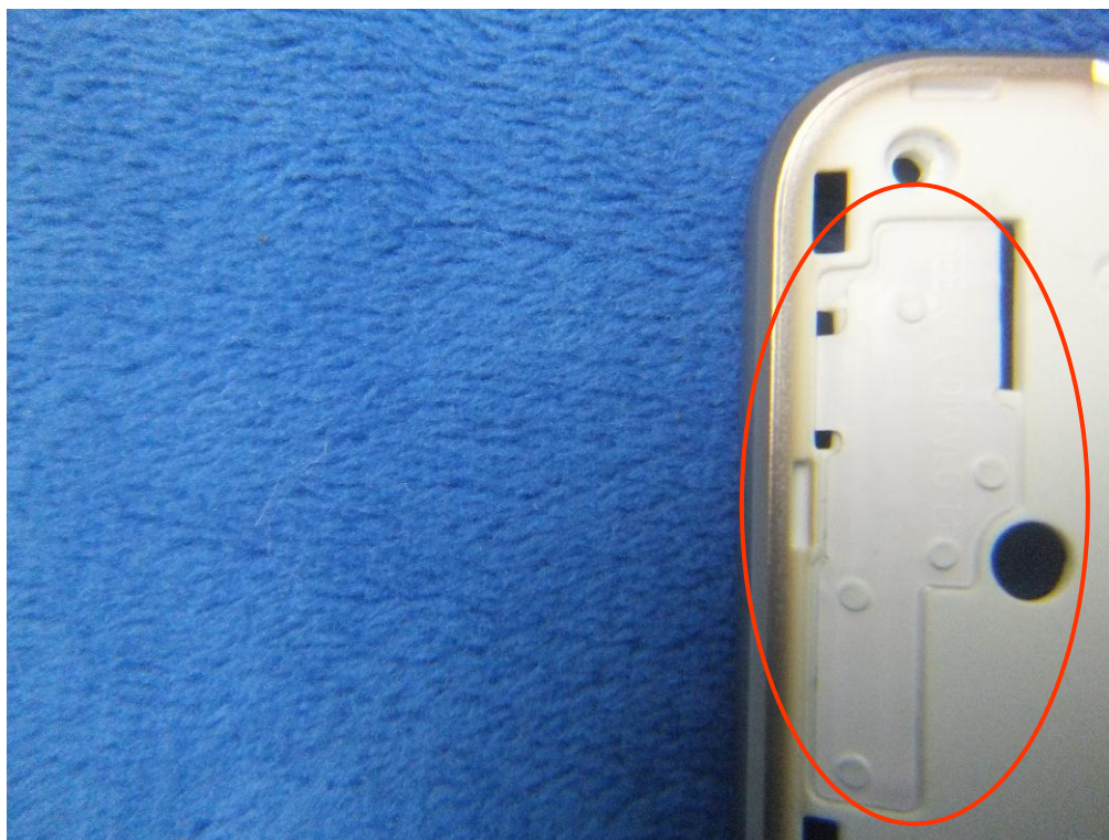
LTE - Antenna View
