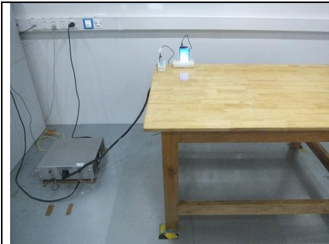
Conducted Emissions Test Setup Front View
