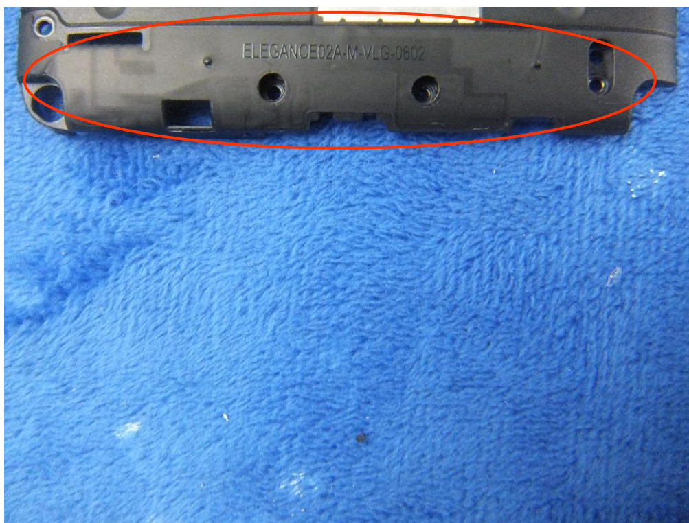
GSM/PCS/UMTS-FDD Antenna View
