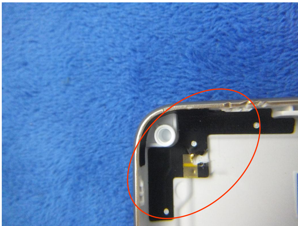
LTE - Antenna View
