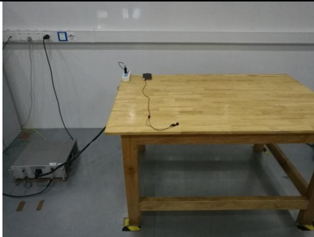
Conducted Emissions Test Setup Front View
