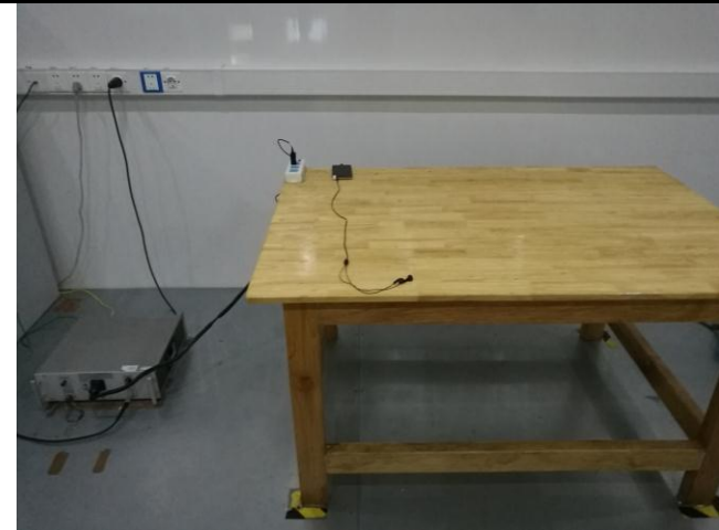
Conducted Emissions Test Setup Front View
