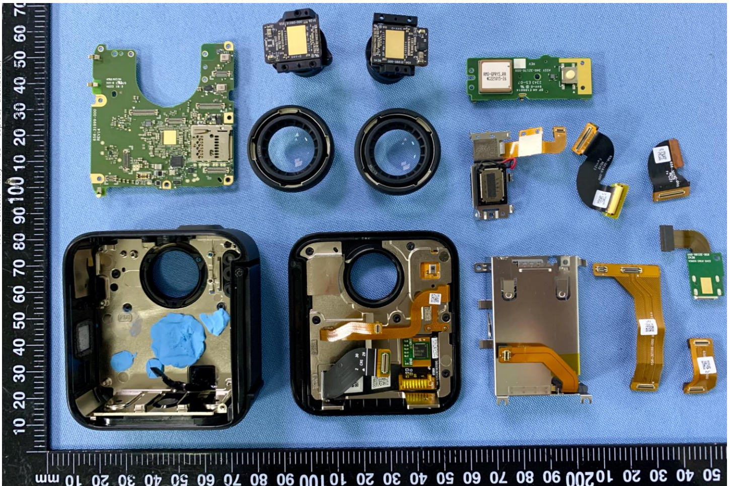
Front/rear cover, battery counterpart, FPCs, USB board, Mic/speaker, GPS board, lens modules/covers, Main board, removed, CPPB1
