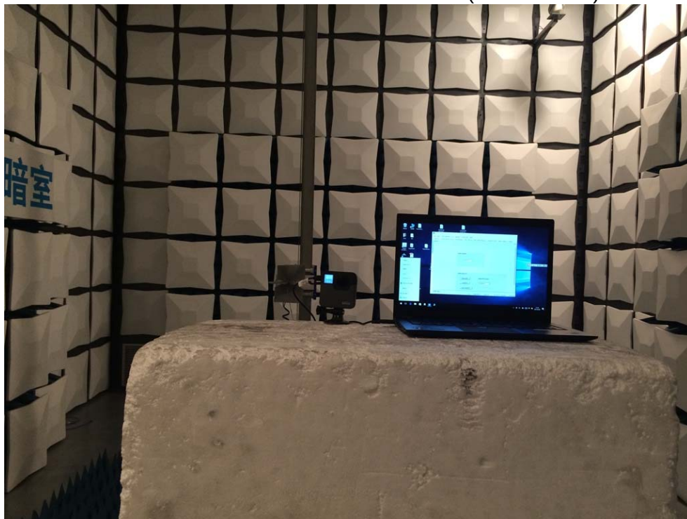
RADIATED RF MEASUREMENT SETUP (Above 1 GHz)
