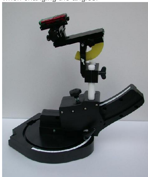
Device holder supplied by SPEAG
