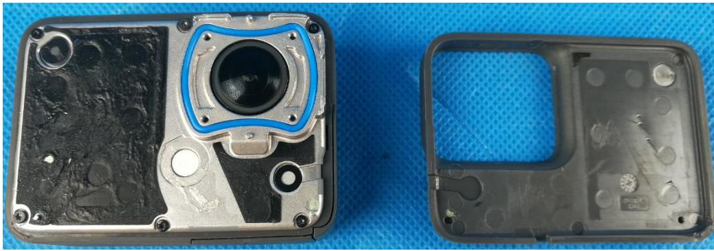
SPTM1 (Version S) front plate removed
