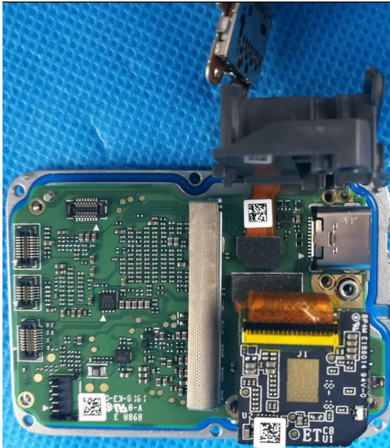
SPTM1(Version S) SD card module removed
