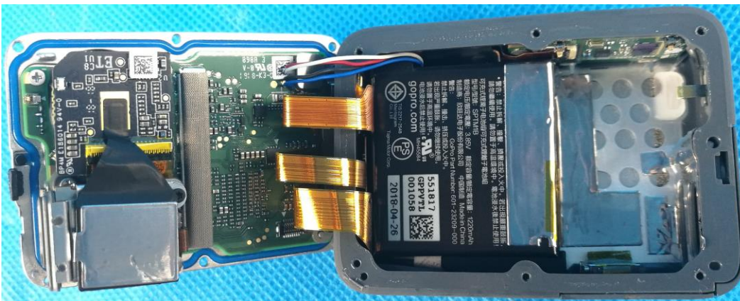
SPTM1 (Version S) heat sink removed
