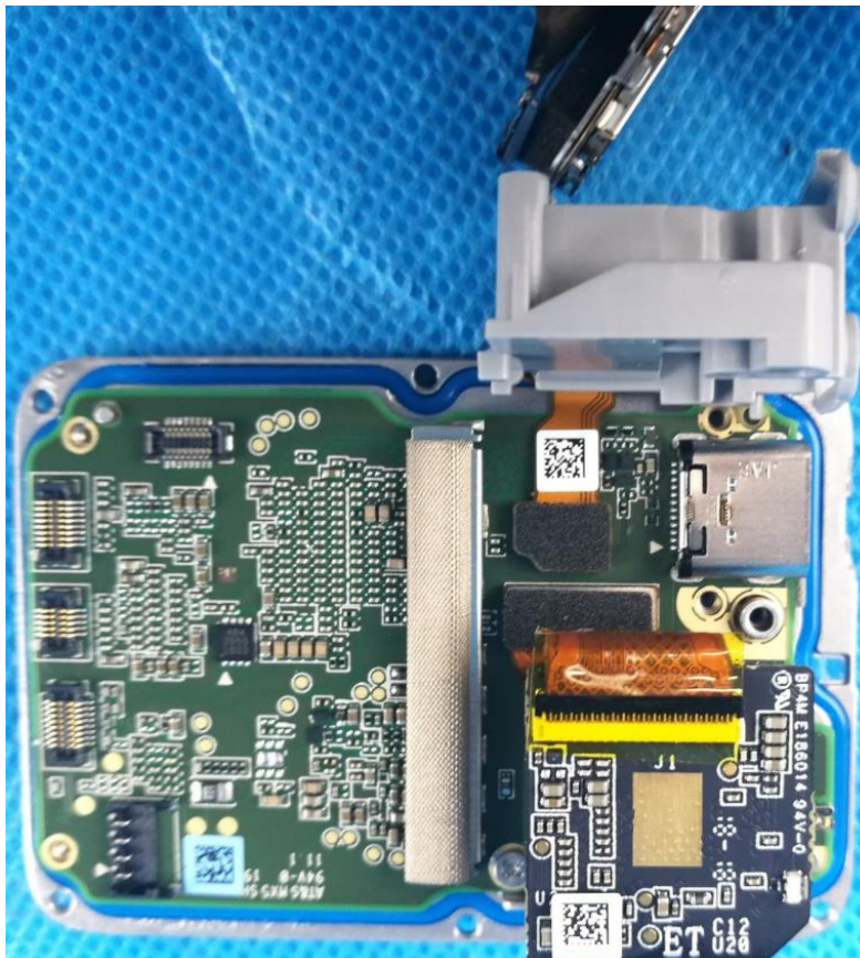
SPTM1(Version W) SD card module removed
