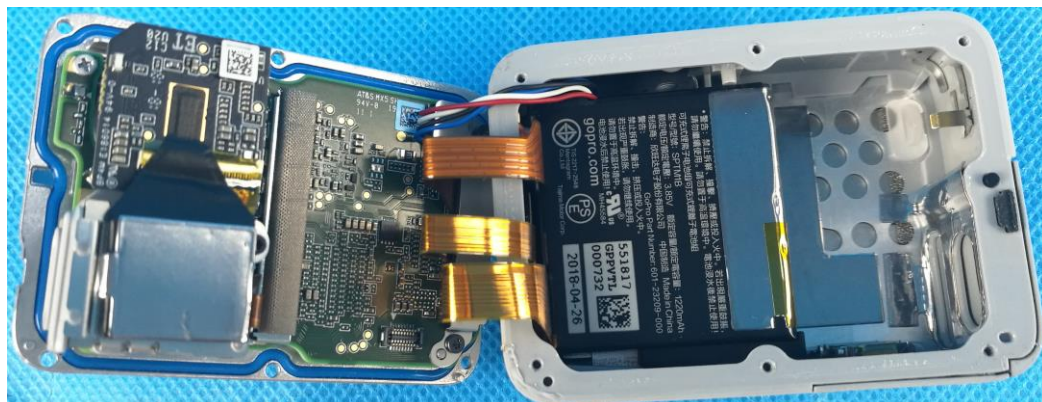
SPTM1 (Version W) heat sink removed
