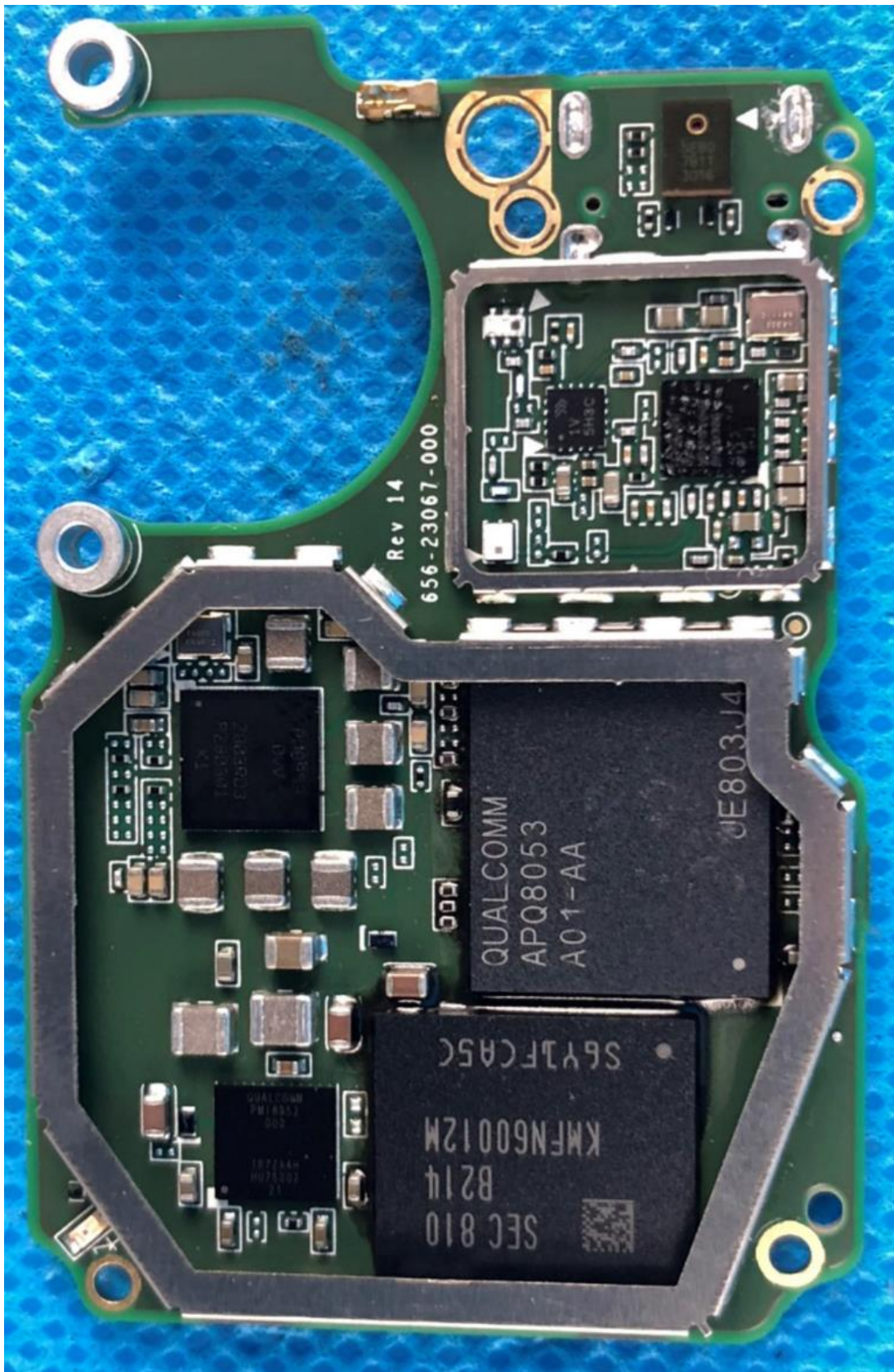
656-23067-000 PCBA, MAIN- SPTM1(Version W)- Front with shield removed
