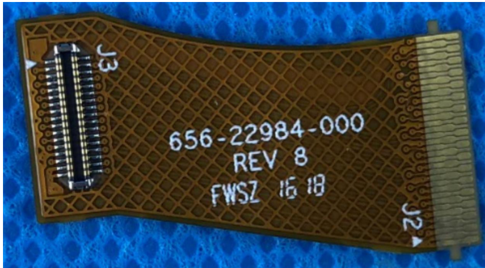
656-22984-000 FPC, JUMPER, IMAGE SENSOR- SPTM1(Version S and Version W) -Front
