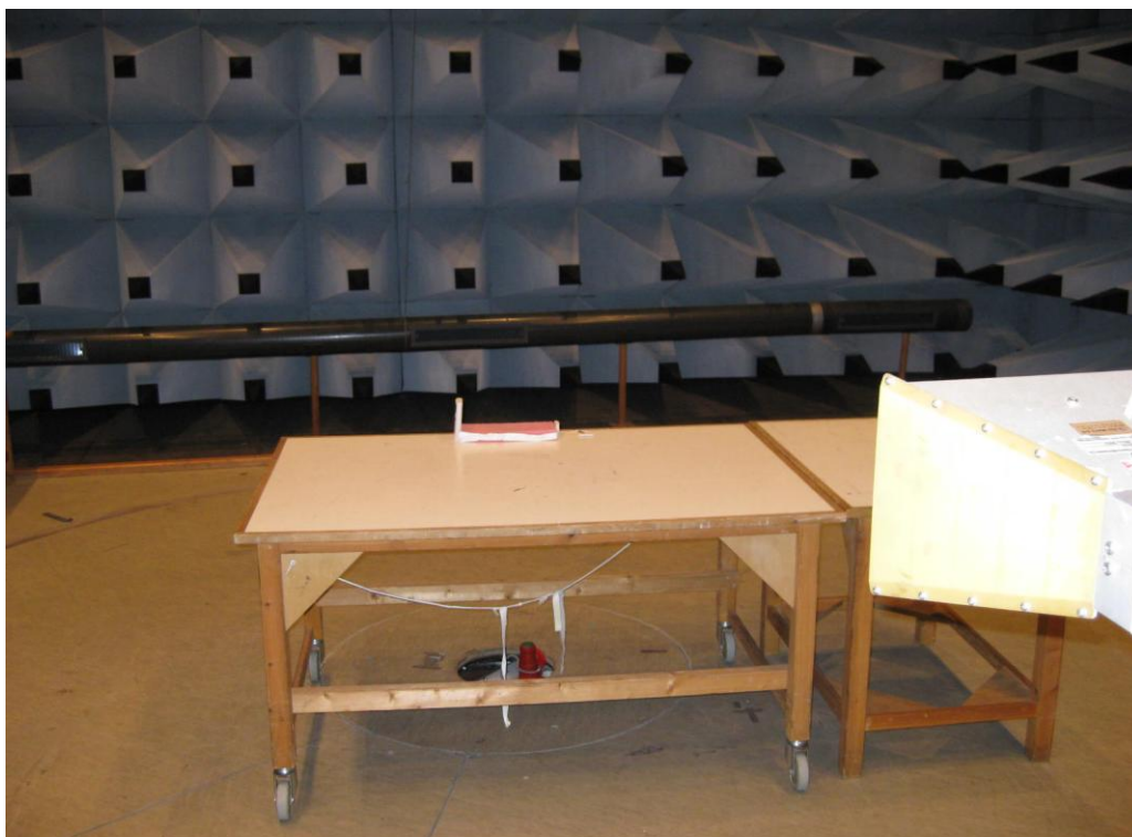
Photo Error! No text of specified style in document..4 Test setup regarding radiated emission, spurious, 1-2.75 GHz.
