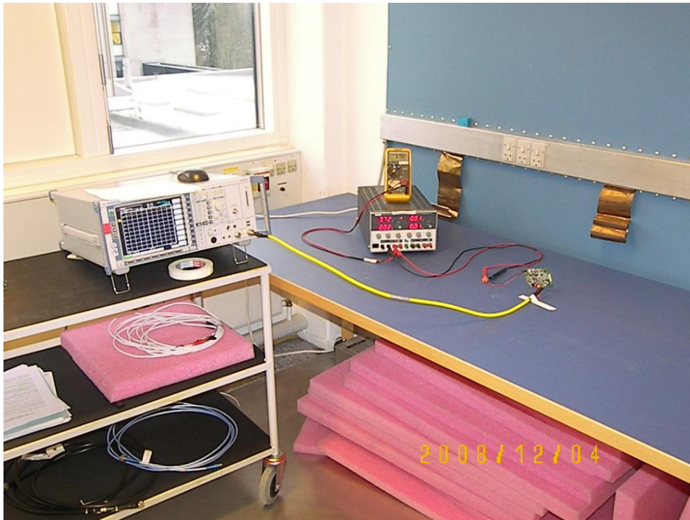
Photo Error! No text of specified style in document..12 Test setup regarding measurement of occupied bandwidth.
