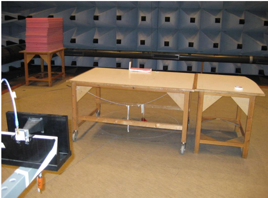
Photo 4.3.7 Test setup regarding radiated emission, spurious, 12.75-18 GHz.
