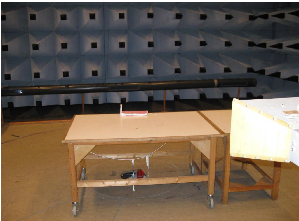
Photo 4.3.3 Test setup regarding radiated emission, spurious, 1-2.75 GHz.
