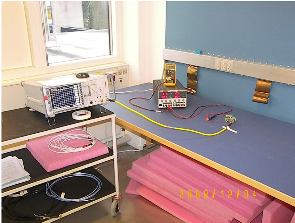
Photo 4.4.1 Test setup regarding measurement of occupied bandwidth.
