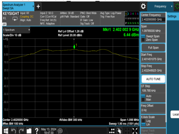
Reference Level BLE 1M MidCH20-2442MHz
