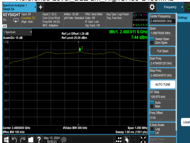
Reference Level BLE 1M HighCH39-2480MHz
