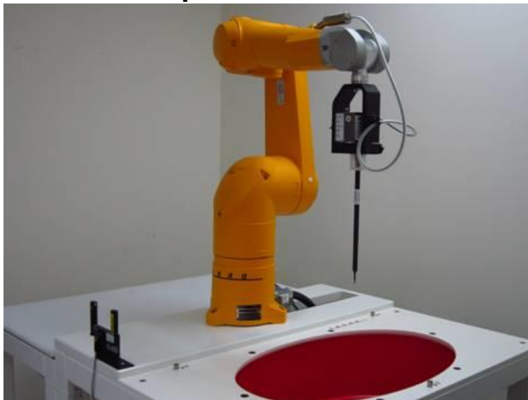
Fig.1 Photograph of the SAR measurement system
