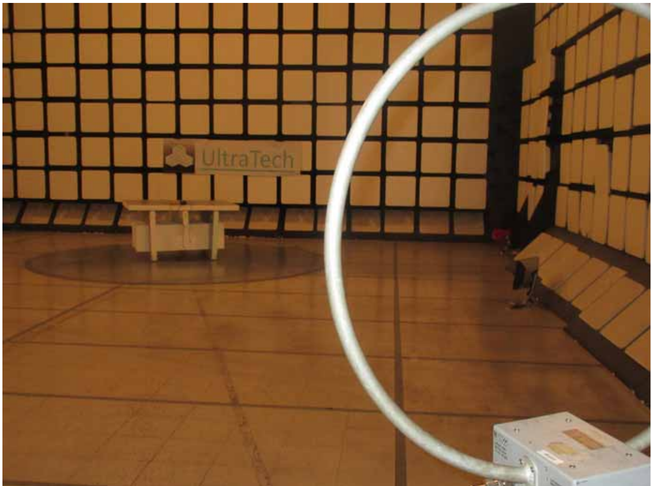
Radiated Emissions at 10 m (Below 30 MHz)
