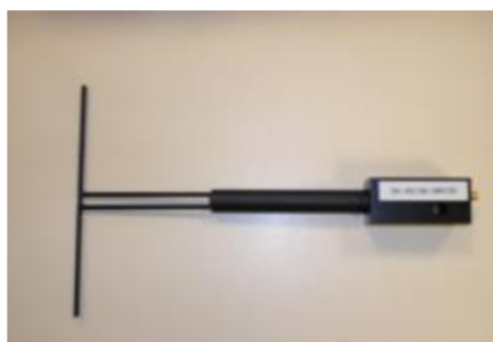
Figure 1 – Satimo COMOSAR Validation Dipole
