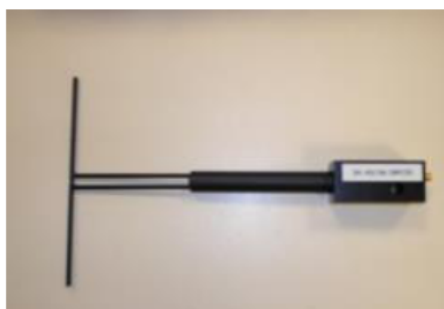
Figure 1 – Satimo COMOSAR Validation Dipole
