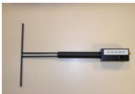
Figure 1 – Satimo COMOSAR Validation Dipole
