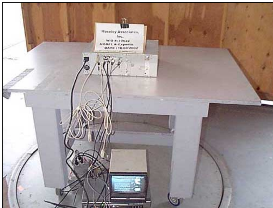
Radiated Emissions - Back View - With UTP Removed
