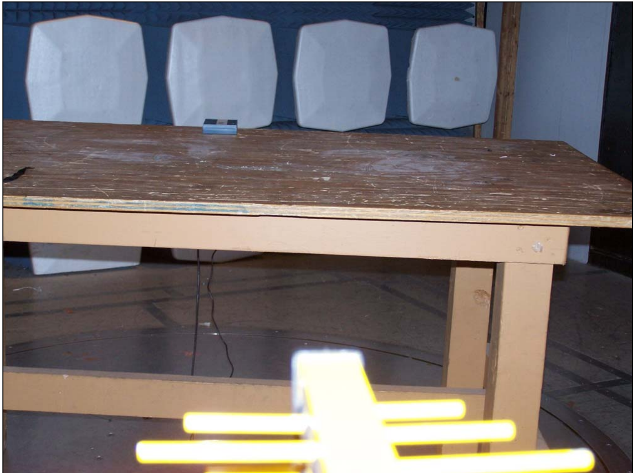
Photograph 4. Unintentional Radiators Test Setup
