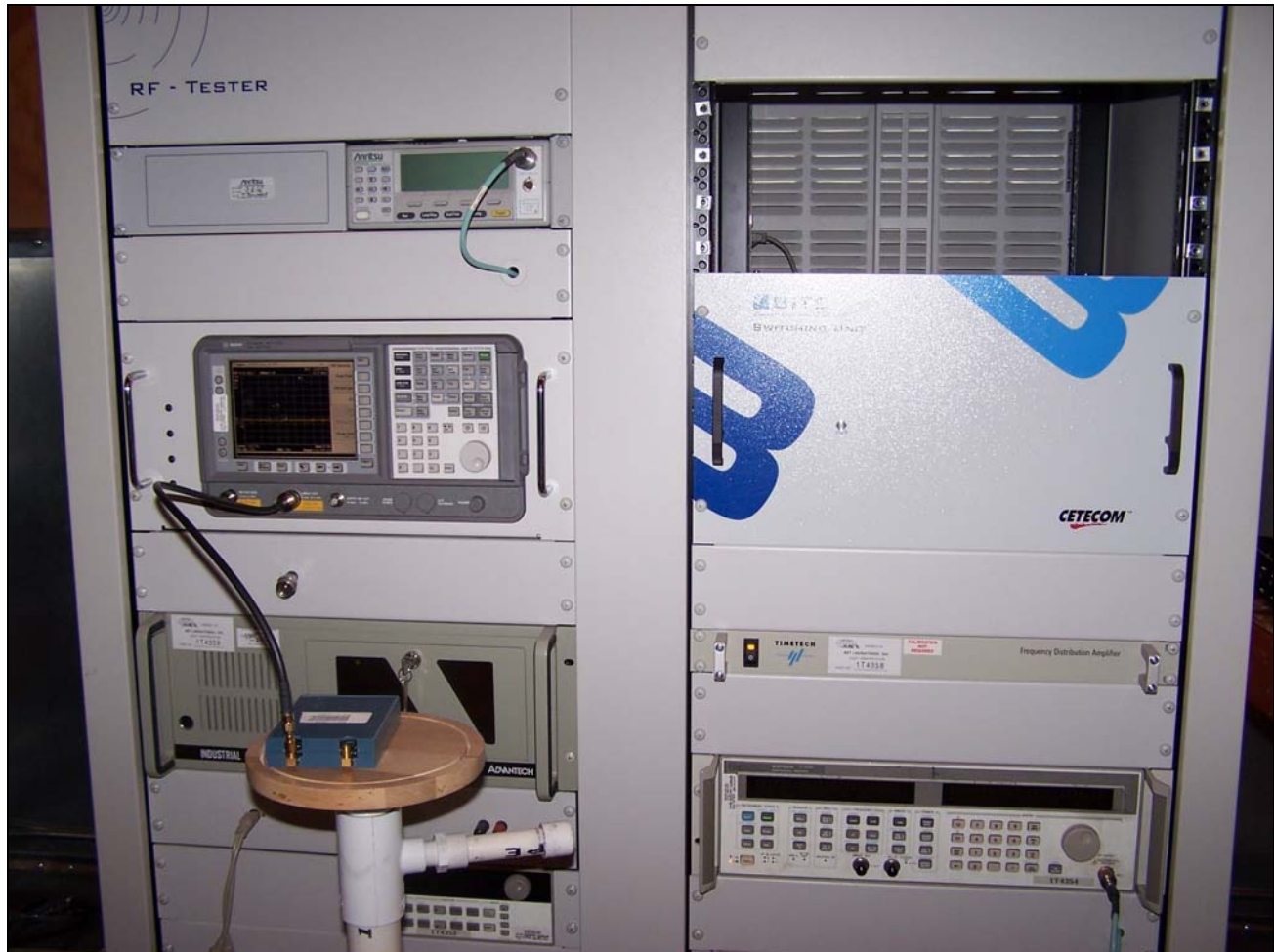
Photograph 5. Power Spectral Density Test Setup
