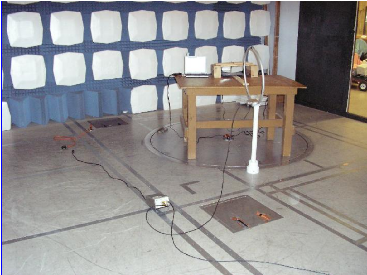
Photograph 3. Intentional Radiated Emissions, Test Setup – Operation at 230 kHz
