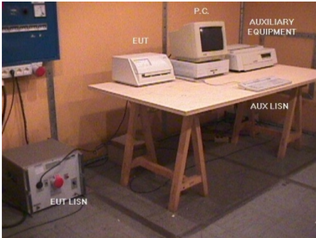
picture 1: conducted measurement front view
