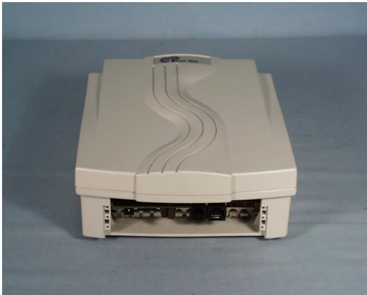
End View of the Four Antenna unit
