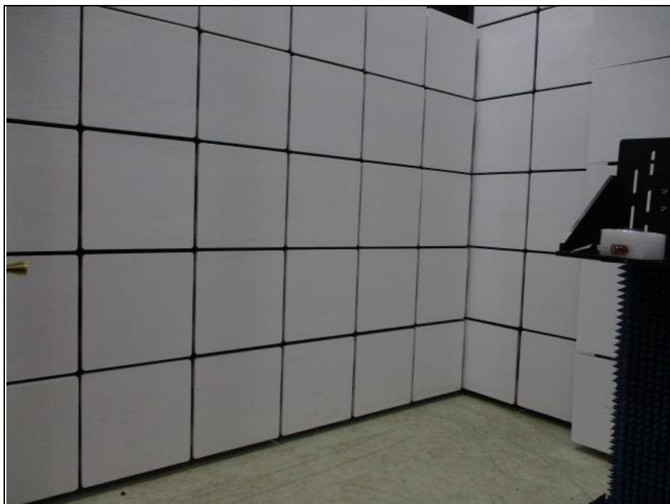
Radiated Emission Test (Frequency range 110GHz ~ 170GHz)
