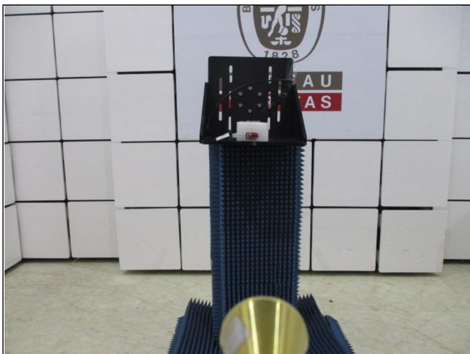
Radiated Emission Test (Frequency range 50GHz ~ 75GHz)
