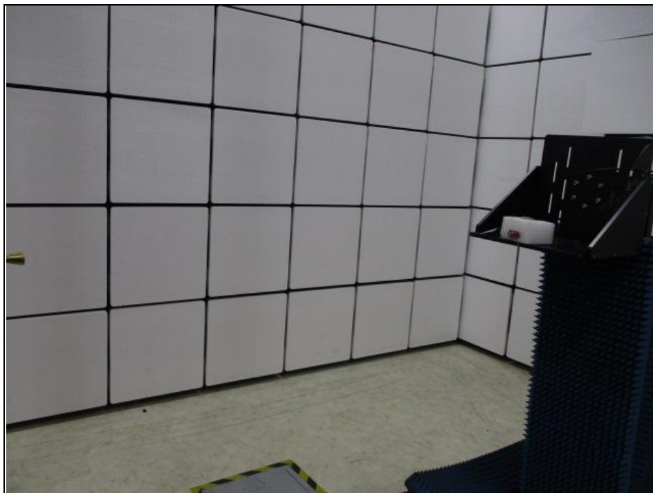
Radiated Emission Test (Frequency range 75GHz ~ 110GHz)
