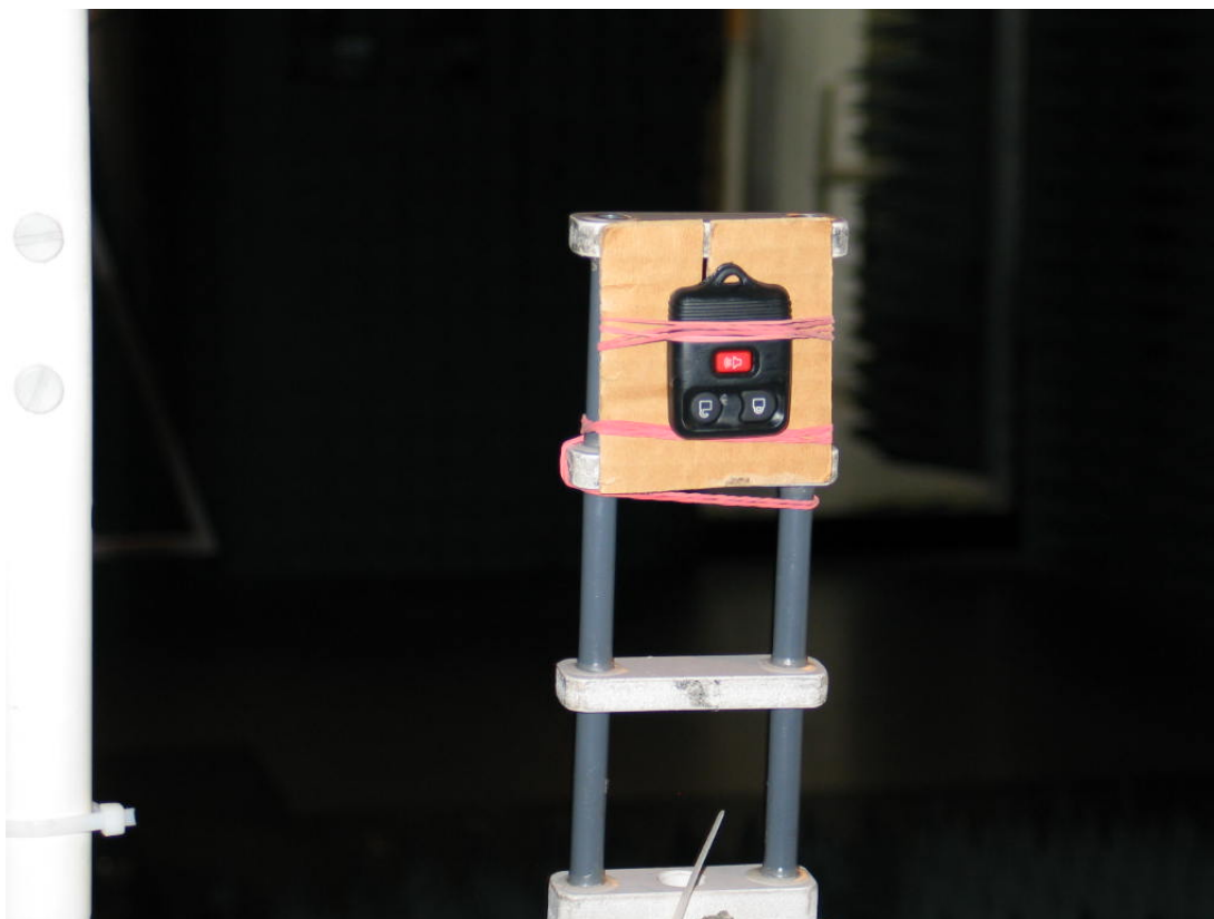
Photo 1: Test setup for radiated measurements
