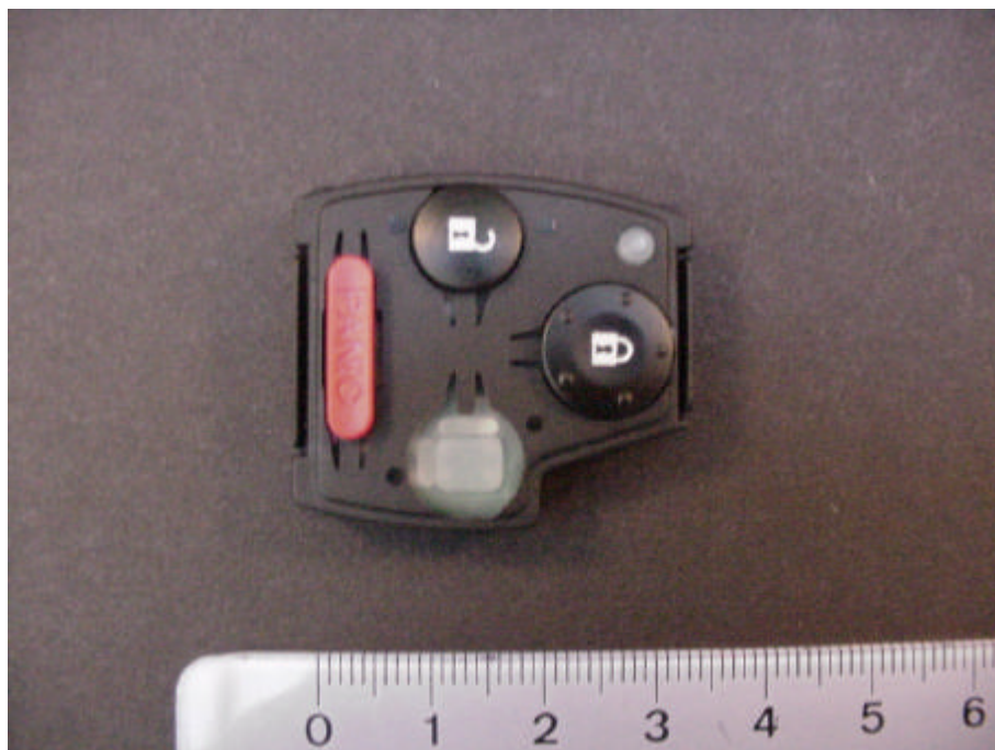
Picture 2 : vehicle remote keyless entry transmitter, inside view, top side
