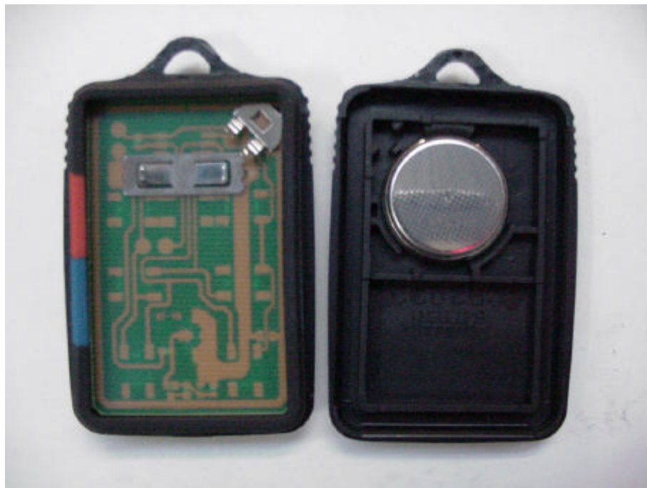
Picture 3 : vehicle remote keyless entry transmitter: 2S4T-15K601-AA, inside view
