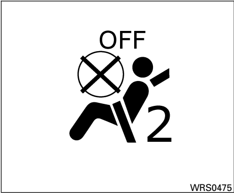
Front passenger air bag and status light
