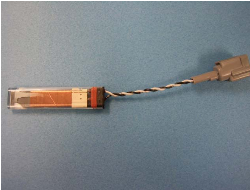
Antenna Internal Photo
