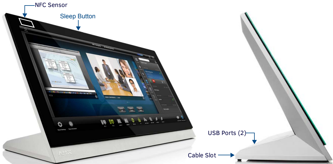
FIG. 6 MXT-2000XL-PAN - Front View
