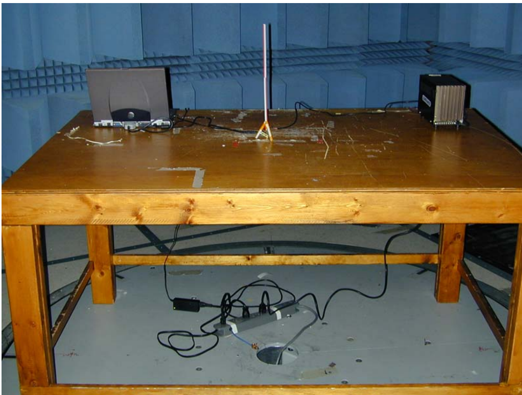
Radiated Emissions at AMD Facility
